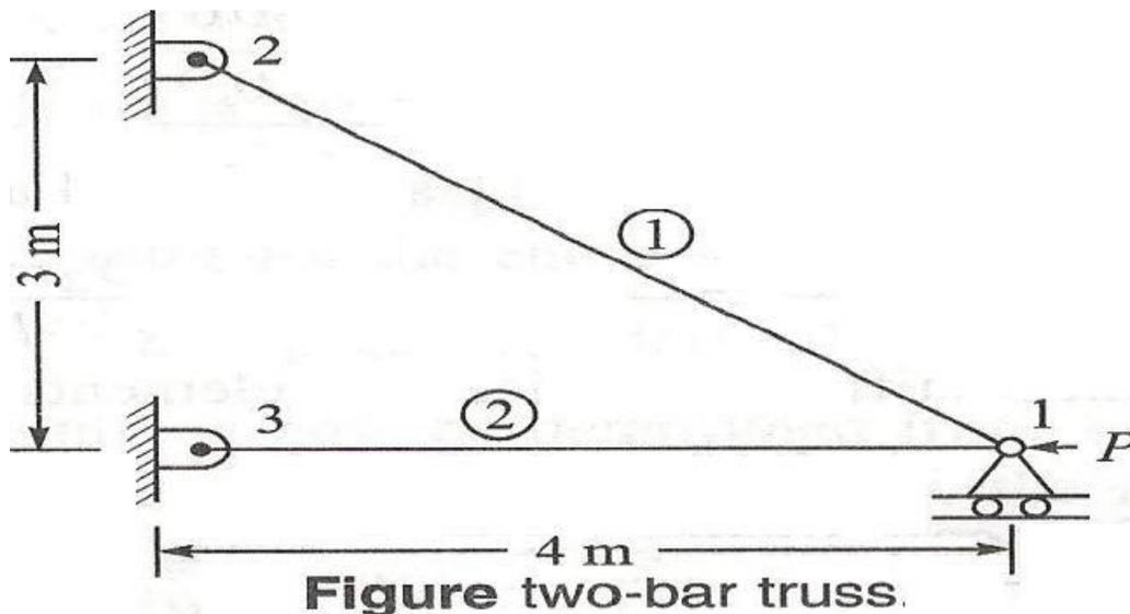
5. Obtain the force in plain truss shown in figure below. And determine the support reactions also. Take  $E=200\text{GPa}$  and  $A=2000\text{mm}^2$ .
