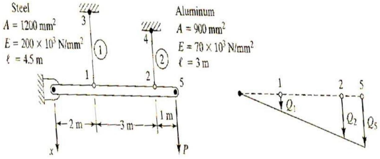
Assemble stiffness matrix and determine nodal displacement for above bar element.
