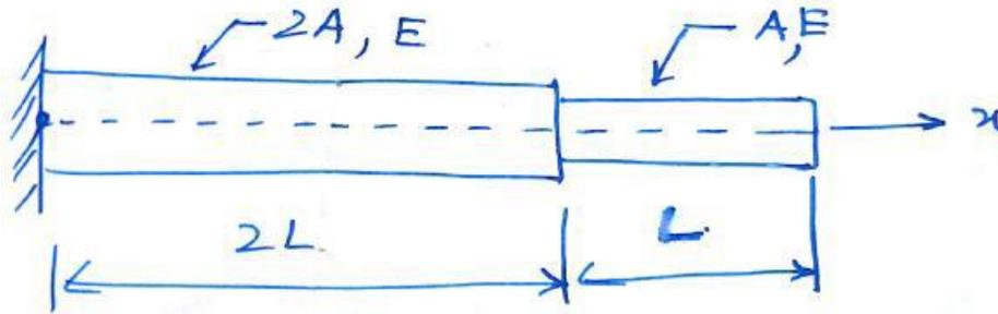
5 . Derive approximate the first two natural frequencies of cantilever beam using one element module.  $EI$ =flexural rigidity.
