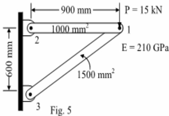
7. Calculate nodal displacements and element stress for the members shown in figure
