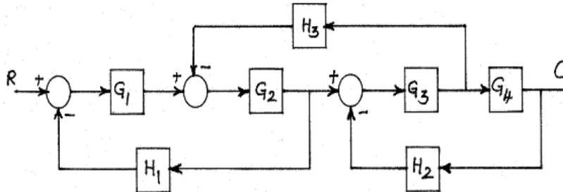
6. Find the closed loop transfer function of the system whose block diagram is given in Fig
