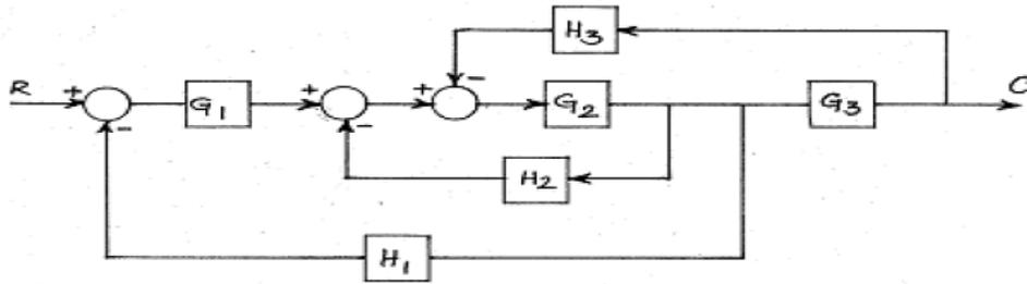
7. Obtain the overall transfer function  $C(s)/R(s)$  of the system shown in figure 2 using block Diagram reduction technique.
