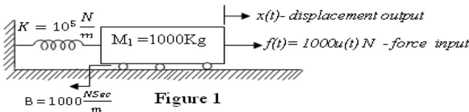
7. Write the governing differential equations of the mechanical system shown in Fig. P1
