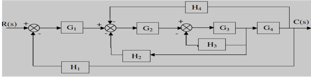
2. Find the overall gain  $C(S)/R(S)$  for the block diagram shown in Figure
