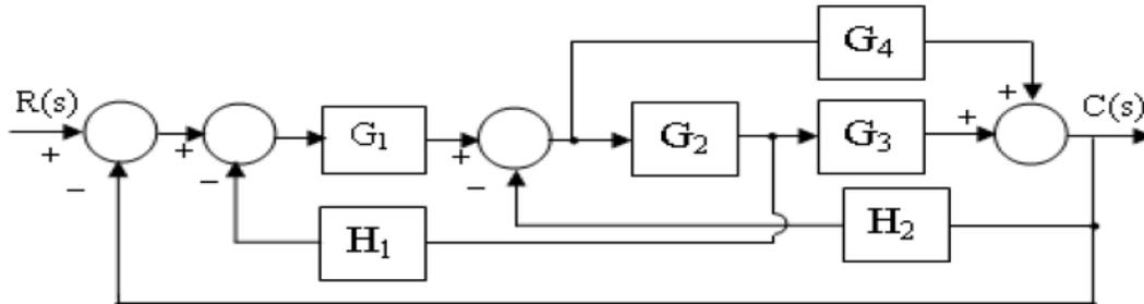
8. Find out transfer function of the following figures by using Signal flow graph rules
