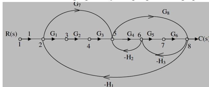
9. Find out transfer function of the following figures by using Signal flow graph rules
