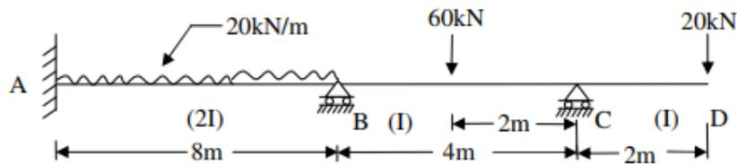
6. Determine the horizontal and vertical component of deflection at the Point 'C' of the frame shown in figure. Take  $E=200 \times 10^3 \text{ N/mm}^2$  and  $I=6 \times 10^7 \text{ mm}^4$ . Use Strain Energy method.
