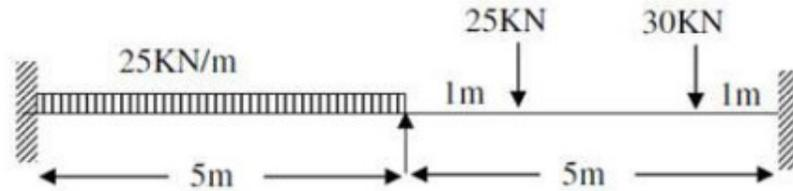
5. Analyse the beam ABCD shown in figure by Slope-Deflection method and draw bending moment diagram.
